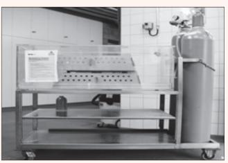
Figure 3 Plastic container, designed to hold several typical rodent transport boxes, linked to CO2 gas bottles.
