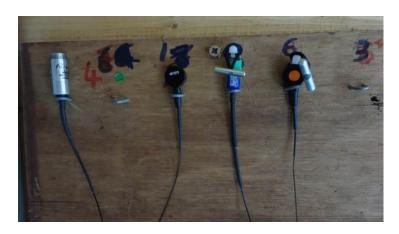
Figure 15 showing a number of different transmitters. The small toggles in this case go through the eyelets on a raptors anklets
