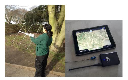
Figures 17 and 18 showing a typical receiver used to locate a transmitter and a new GPS system that links with GPS technology in smart phones and tablets.
