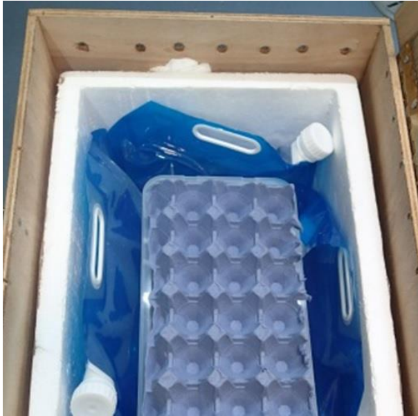
Water bags surrounding inner Partula container with egg carton on top to facilitate air flow to inner container
