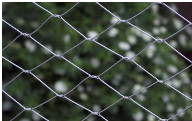
Fig. 9 Woven mesh with interwoven cables
