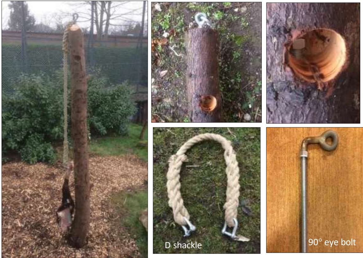
Set up and components of the swing ball enrichment device at Chester Zoo.
